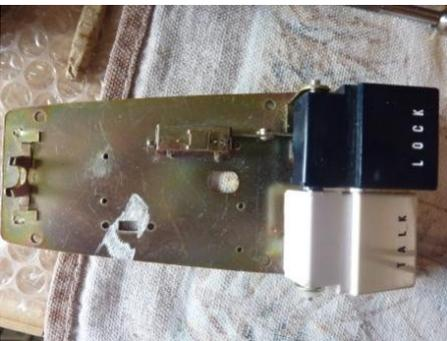
The PTT- in fact there are two, one conventional with a lock and the other on the base that is actuated by lifting the mic. The American Hams will like this, so they thought, but quite often you find the wires to this cut so clearly it was an annoyance to some.
