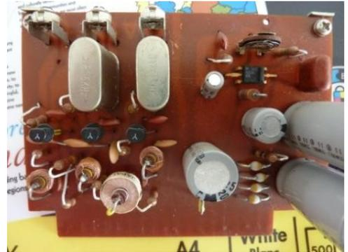
The first time I encountered this problem, it was after prolonged use on a hot Summer's day, the receiver just died and the VFO led went out. The Yaesu manual did not have a schematic -it did show the pcb's but the regulator board shown did not match the one in my set- I made the assumption that there was a voltage line missing and so went straight for the regulator board.
