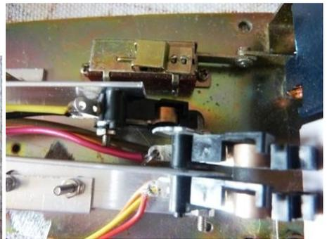
At this point I should say that the YD844A was a dual impedance mic, but as the mic element was missing, the hunt started for a suitable replacement. The covering of the impedance selector switch by the new brackets was unimportant as this was never going to be a restoration in the true sense- more of a rebuild from scratch.
