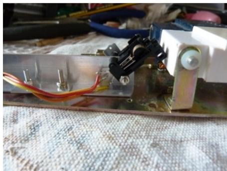
A piece of aluminium formed and drilled to suit existing holes in the base plate will be the answer and it was a case of offering the bracket and switch to the PTT button and adjusting for reliable operation.
