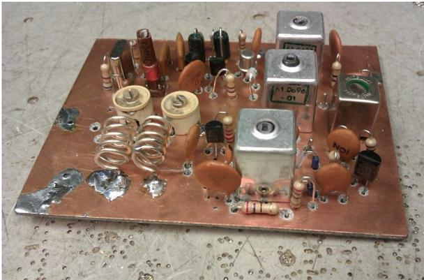
The down converted IF leaves the mixer and is fed to a HF ( 28 - 30 MHz ) grounded base preamp Tr2. The local oscillator strip uses a 38.6666 MHz third overtone xtal multiplied by X3 to produce a LO frequency of 116 MHz. With a average sensitivity HF receiver this 2m con-
