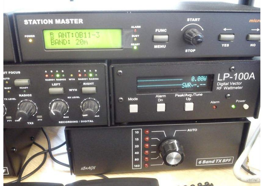
Picture of power / SWR meter. The Station Master unit above it controls the antenna switch.
