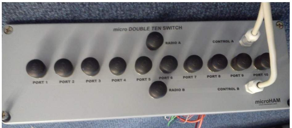
*Picture of the front of the switch. Two coax connections for the two radios, two control lines for the two radios, and then coax connections for the antennas.*
