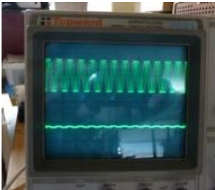
At 700Hz no output to the tweeter
