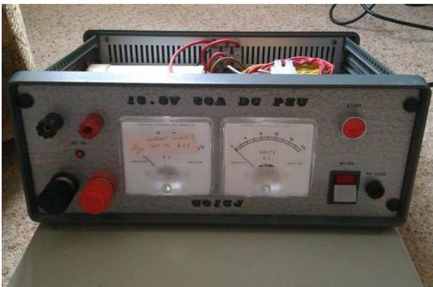
trolled over-voltage shutdown, this heavy-weight is designed to protect your rig should a fault develop.
