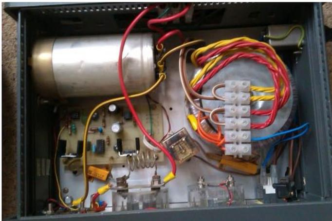
This latter difference is more important than it first seems as there is a potential safety issue here. The soft start relay carries full mains voltage on its contacts and placing it on the pcb gives a risky mix of full mains and 12v dc on the same board where a slip of a probe or finger could give unpleasant results.
