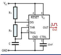
The frequency of the square wave is determined by the components R1, R2 and C. In the Vellerman kit R1 = 1k, R2 = 15k and C = 47nF and this gives an approximate 1kHz square wave.
