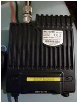
type of connector it has to be said especially where continual flexing is likely as for the fist mic during use, but par for the course on rigs at this price point. The DC lead in in two parts, connected via a standard two way spade coupler. A line fuse in the red lead of both halves is a bit odd and does seem to cause a slight voltage drop during transmit on full power.
