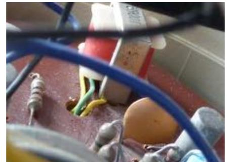
Short cleared but results were still horribly distorted, so back to voltage checks. All voltages around the output transistors were too far off those on the circuit and therefore I deduced that both output devices were damaged. A couple of Mullard pnp types were popped in temporarily but would you believe it, still distorted audio.
