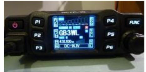
"read" the radio before the first install of data. 200 channels are available to the user and all the usual functions are available within the software. Once the programming is done, the mic can be connected, button P2 toggled to Memory and off you go!
