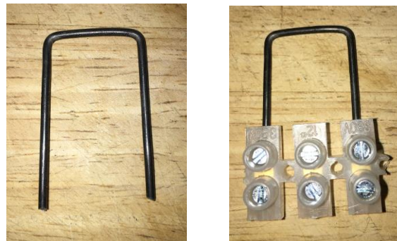
Fold short lengths of wire with a pair of pliers
