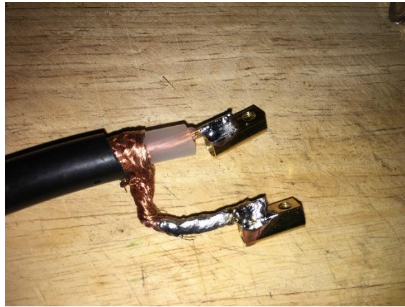
Solder the inserts as shown. Note one screw hole on each is uncovered.
