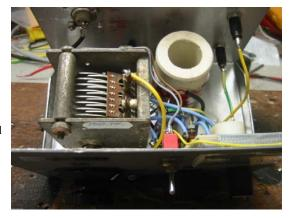
Screened coaxial cable should be used for the RF connections to and from the SWR bridge. Keep wires going to the switch from the coil as short as possible. The variable capacitor in the L match can be from 150 to 200pf, use wide spaced if using powers above 10 Watts. An SO239 socket was used for the input to the RF input to the unit and Banana sockets for the antenna and ground connections. The ATU should be mounted in an RF tight enclosure. The T68-2 torroid is available from the G-QRP club.
