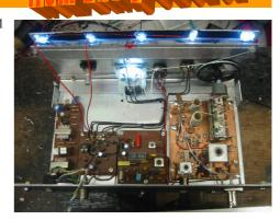
simple circuit it really does perform well, you could use a more elaborate circuit with better performance but I don't think it is justified in this project. All of the transistors used are BC108's (Europa again!), however any general purpose npn small signal transistor will do (BC546 etc.)
