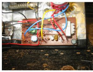
load for Tr2, so no RF will pass through the transformer, AUDIO frequencies however will and do pass freely via the transformer to the secondary winding. So, audio is present at the secondary of T1 at a source impedance of very roughly 500 Ohms. This source impedance is not low enough to drive the low impedance headphones (40 ohms or so) to a useable level; a further impedance transformation is needed.
