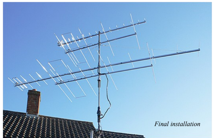
New rotator and bearing fitted then 432/70MHz fitted on mast
