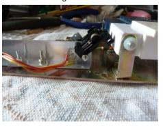
A piece of aluminium formed and drilled to suit existing holes in the base plate will be the answer and it was a case of offering the bracket and switch to the PTT button and adjusting for reliable operation.
