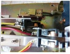
At this point I should say that the YD844A was a dual impedance mic, but as the mic element was missing, the hunt started for a suitable replacement. The covering of the impedance selector switch by the new brackets was unimportant as this was never going to be a restoration in the true sense- more of a rebuild from scratch.
