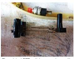
The original PTT switches were large with long leaves which seemed to go out of shape and indeed the one that remained looked reasonably OK but failed miserably to make contact. Two sessions with the sonic cleaner cleaned up the leaves but contact was unreliable and so a modern solution was needed.
