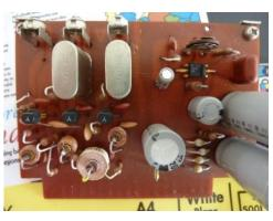
The first time I encountered this problem, it was after prolonged use on a hot Summer's day, the receiver just died and the VFO led went out. The Yaesu manual did not have a schematic -it did show the pcb's but the regulator board shown did not match the one in my set- I made the assumption that there was a voltage line missing and so went straight for the regulator board.
