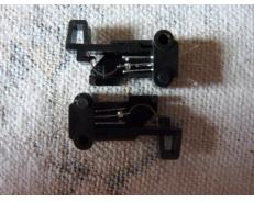
Two types nearly made the grade but were finally discounted as I could not reliably achieve sufficient lever movement to actuate the switch.
