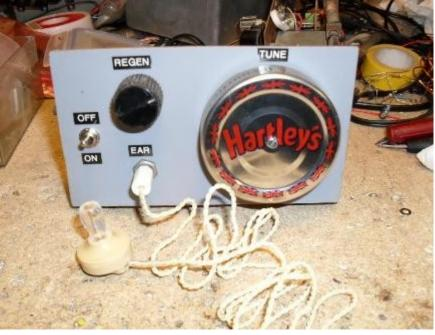
RF stages are operating at the incoming signal frequency, unlike a superhet which converts the incoming RF signal to a fixed frequency (Intermediate Frequency) and it is this IF frequency where the bulk of selectivity and gain is achieved.
