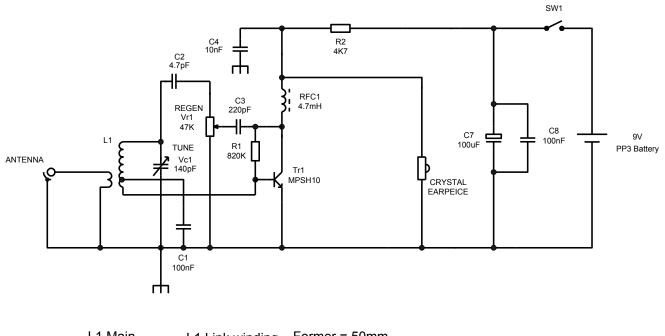
L1 Main winding = 25 turns 30 swg enamelled copper wire, tap at 3 turns from ground end
