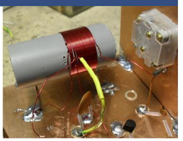
oscillation ( this will sound like a squeal / hissing sound in the earpiece ). For SSB reception bring the set to "almost" oscillation, CW reception requires slightly more regeneration. The tuning of SSB and CW stations will be very sharp and requires practice, a large control knob on the tuning capacitor is recommended.
