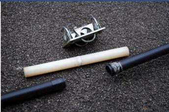
10m band, from centre of dipole centre to ends of the wire: 2.49m 15m band as above 3.33m
