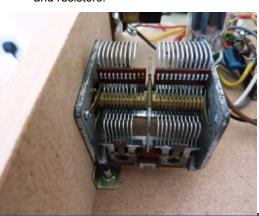
durable compost heap proof radios- and after three cycles through the sonic cleaner and one hour at 50 degrees C in the oven, the tuning capacitor measures spot on for this project.
