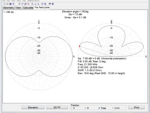
around to build a fan dipole for 10m and 15m. I wondered if the "fan" in fan-dipole was a myth? I thought about placing the 10m elements on one side of the fishing pole and the 15m elements on the other side, about a 25mm
