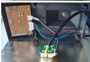
G4VPD came back and said it sounded fine. Job done so I postioned the little preamp pcb on some double sided tape on the metal base plate and re-assembled the mic. Result happy G0EYO. Anyone want to buy a fist mic?
