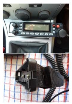
I decided therefore to mount the removable head in a space just in front of the manual gearchange and home brewed a piece of wood to fit which gave me a
