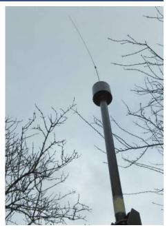
was working well with good signals on all HF bands and no cross modulation effects. At this Voltage it was drawing about 50mA from the power supply. My supply will actually produce 33V so I gave it a burst of that and the current increased but there was no change in performance, so I returned it to 24V.
