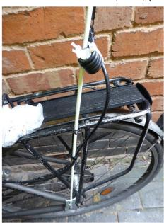
to form a choke. The radiator is just a random piece of coated multi-strand wire from the junk box, but I use ladder line for the stub. Some designs on the web suggest using ladder line for the whole thing, but this can make it a bit more costly. Multi-strand wire is also easier to roll-up if the j-pole is for portable work, not the bike!
