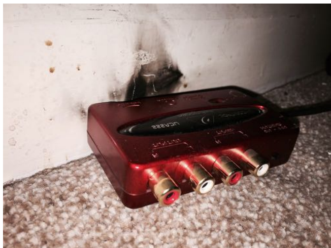
Where lightning leaked magic smoke from USB sound interface against skirting board
