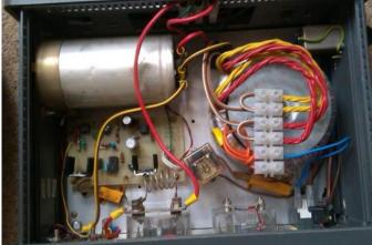
As for the second one, it was clear that the soft start relay was not latching and therefore the power supply was not starting. The relay was a rather chunky octal based 24v two pole changeover type which was pulled from its very tight socket. The pins looked clean and so I reinserted it.
