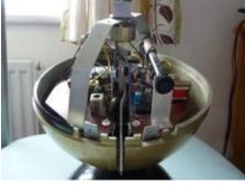
Digging deeper in the RF part, I found the alignment to be way out, so with that corrected reception was as expected through my bench amplifier.
