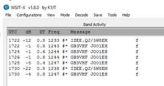
You can deal with this by going to the box to the left of the frequency display on the decoding screen, and select 144.120MHz'.
